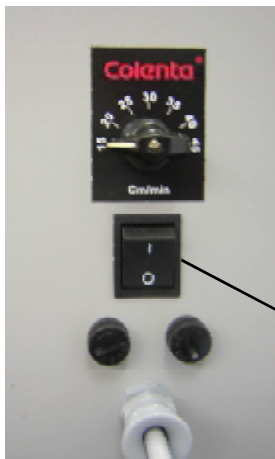
Main power switch
